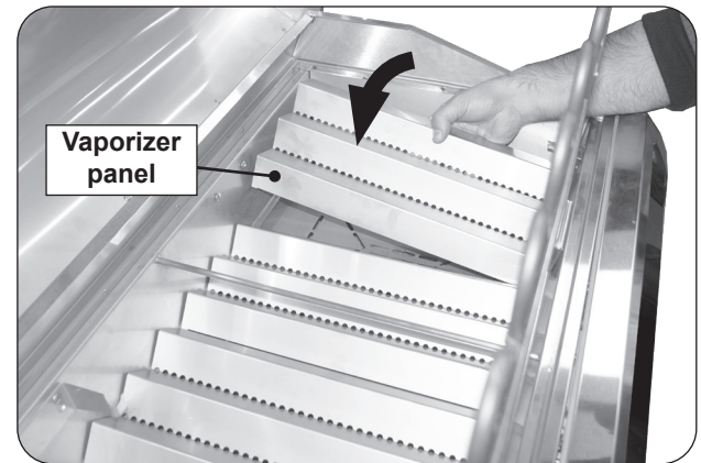
Fig. 25-2 Install vaporizer panels
