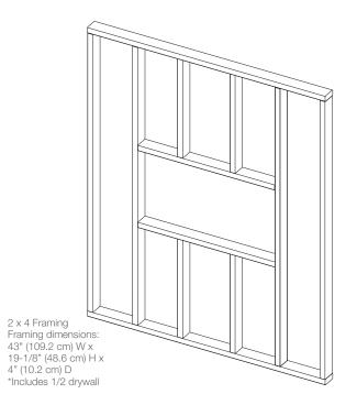
The Firebox is not load bearing. Do not stack weight of the frame on top of the firebox.
