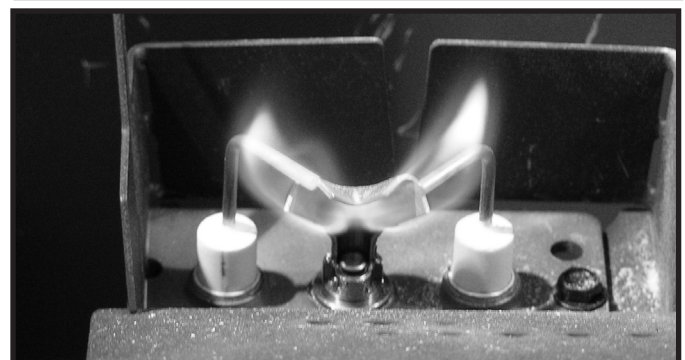
Figure 4.2 IPI Pilot Flame Patterns
