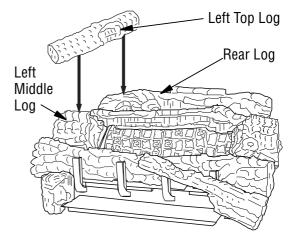
Figure 32 - Installing Left Top Log
