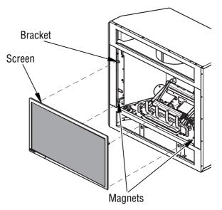
Figure 38 - Installing Fireplace Screen
