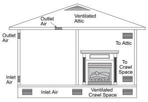
Figure 4 - Ventilation Air from Outdoors
