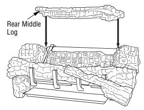
Figure 30 - Installing Rear Middle Log
