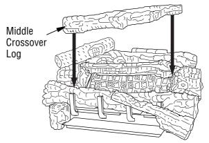
Figure 33 - Installing Middle Crossover Log
