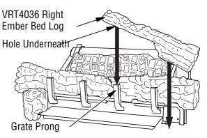
Figure 27 - Installing Right Ember Bed Log
