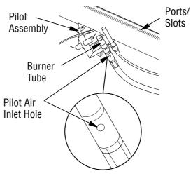
Figure 46 - Pilot Inlet Air Hole
