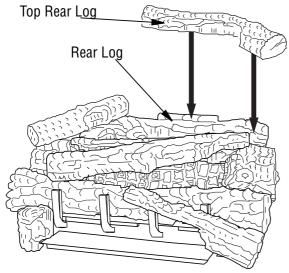
Figure 34 - Installing Top Rear Log
