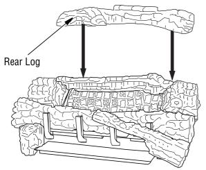
Figure 31 - Installing Rear Log
