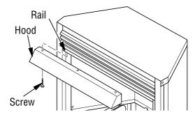
Figure 5 - Installing Hood
