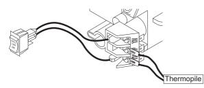
**CAUTION:** Label all wires prior to disconnection when servicing controls. Wiring errors can cause improper and dangerous operation. Verify proper operation after servicing.
