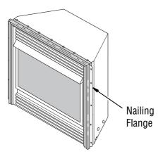
Figure 11 - Location of Nailing Flange
