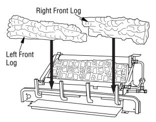
Figure 25 - Installing Left/Right Front Logs
