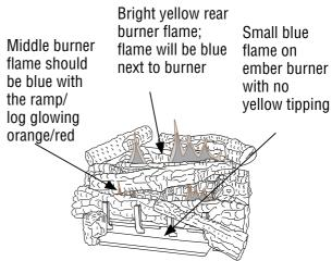
Figure 43 - Correct Burner Flame Pattern
