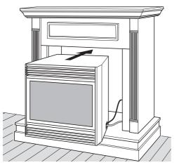
Figure 12 - Inserting Fireplace Into Cabinet Mantel
