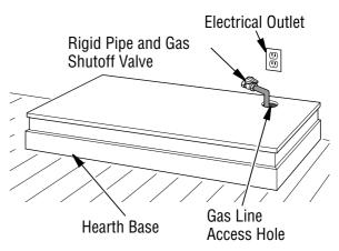
Figure 9 - Placing Hearth Base Accessory Against Wall
