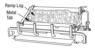
Figure 24 - Installing Fiber Ramp Log
