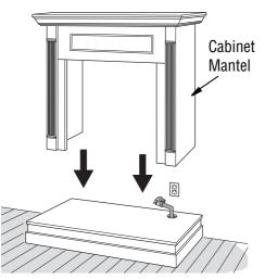
Figure 10 - Installing Cabinet Mantel
