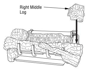
Figure 29 - Installing Right Middle Log
