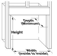
Figure 13 - Rough Opening for Installing in Wall
