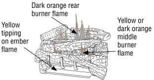
Figure 44 - Incorrect Burner Flame Pattern
