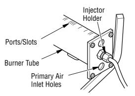
Figure 45 - Injector Holder On Outlet Burner Tube
