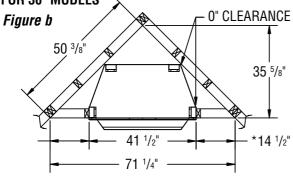
\* THESE DIMENSIONS ALLOW FOR MINIMUM CLEARANCES TO A 45° PROJECTED SIDE WALL
