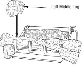
Figure 28 - Installing Left Middle Log
