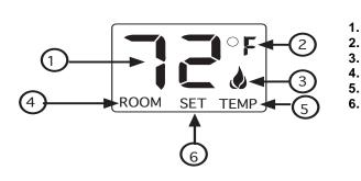
DISPLAY Indicates CURRENT room temperature. °FOR°C Indicates degrees Fahrenheit or Celsius. FLAME Indicates burner/valve in operation. Indicates remote is in THERMO operation. Appears during manual operation. Appears during time the of setting the desired temperature in the thermo operation.
