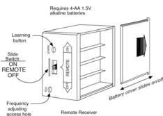
Make sure the remote receiver switch is in the OFF position. It is recommended that 18 gauge solid or stranded wires (included) be used to make connections between the terminal wiring block on the millivolt gas valve or electronic module and the wire terminals on the remote receiver. For the best results, use 18 gauge stranded wire, with no splices and measuring no longer than 20 ft.
