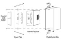
Position the cover plate so the word ON is facing up; then, install the remote receiver into the plastic switch box using the two long screws provided. Push the White Button over the receiver slide switch only
