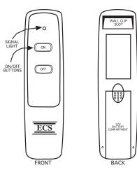
The transmitter operates on a 12V battery (included) made specifically for remote controls and electronic lighters. Install the 12V battery supplied with the unit into the battery compartment.
