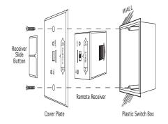
NOTE: The remote receiver will only respond to the transmitter when the 3-position slide button on the remote receiver is in the REMOTE position. If the system does not respond to the battery transmitter on initial use, see MATCHING SECURITY CODES, and recheck battery positions in the remote receiver.
