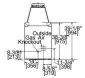
Framing dimensions in illustrations accommodate 1/2" finishing material.
