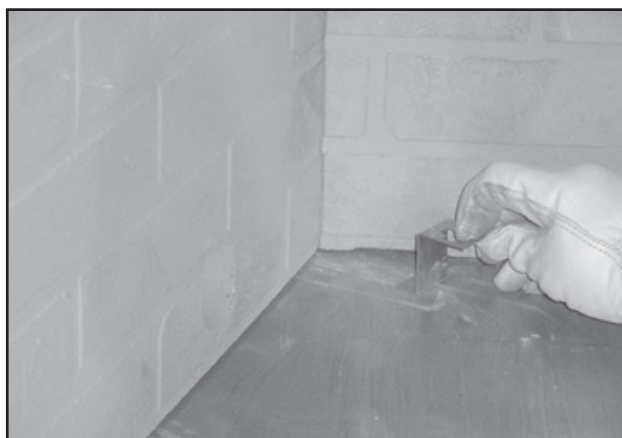
Figure 8.7 Slide Grate Retaining Bracket into Notch
