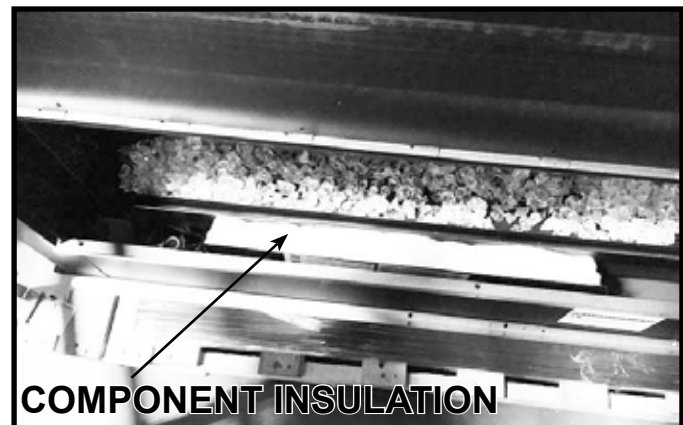
Figure 11.3 Component Insulation Location
