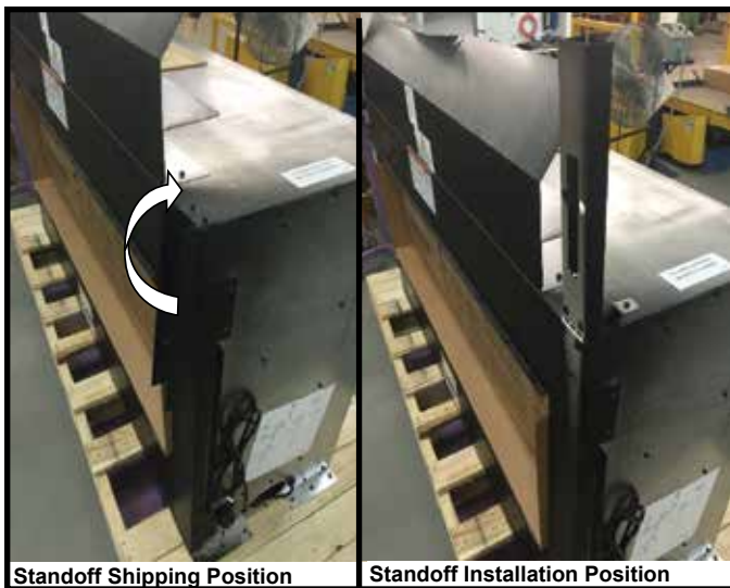
Figure 6.1 Standoffs Shown in Vertical Position
